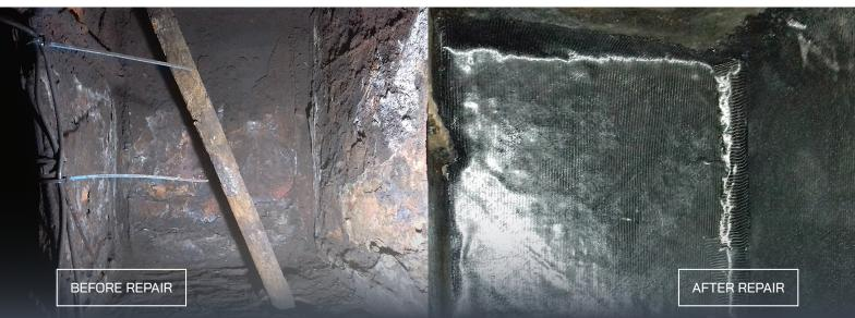
The floor and the bulkhead plates in ballast tank were corroded and HFO was leaking into the sea water through the plates. The repair was conducted during the vessel's voyage that lasted 3 days.
